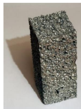
Figure 1.3. Photography of a block of aluminum foam.
