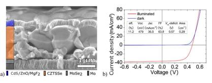
**Figure 5.** (a) SEM cross section exhibiting large grained morphology and (b) dark and illuminated current density-voltage (J-V) measurement of the 11.2% efficient solution processed kesterite solar cell treated with NaCl. Reprinted with permission from [41]. John Wiley & Sons. (© 2015 WILEY-VCH Verlag GmbH & Co. KGaA, Weinheim).
