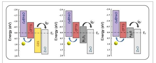
Figure 15. Schematic energy level diagram of CFTS/CdS, CFTS/Bi $_2$ S $_3$ , and CFTS/Ag $_2$ S heterojunctions. The line at 0 V represents the Fermi energy after contact. Reprinted from [160]. Copyright (2017), with permission from Elsevier.
