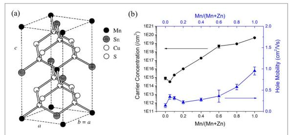
Figure 14. (a) Crystal structure of Cu<sub>2</sub>MnSnS<sub>4</sub>. Reprinted (figure) with permission from [139], copyright (1997) by the American Physical Society, (b) carrier density as a function of Mn/(Mn + Zn) in CMZTSSe. Reproduced from (2017) with permission of The Royal Society of Chemistry.
