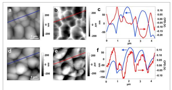
Figure 4. AFM topography images (a), (d), Scanning Kevin probe microscopy (SKPM) potential maps (b), (e) and. plots of the topography and potential linescans (c), (f) (a)—(c) of CZTSSe films without (a)—(c) and with Li-doping (d)—(f). Reproduced from [23] with permission of The Royal Society of Chemistry.
