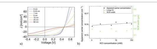
**Figure 6.** (a) J-V curves of KF-PDT treated solution processed kesterite solar cells that exhibit increased blocking of the  $J_{SC}$  with thicker KF layer (0 nm–60 nm). Reprinted from [47], Copyright (2017), with permission from Elsevier. (b) Increase of the apparent carrier concentration as determined by C-V measurements on bulk treated solution processed kesterite solar cells. Copyright © 2018, Author(s). Reproduced from [48]. CC BY 4.0.
