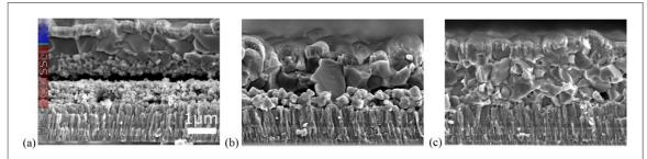
Figure 7. SEM cross sections of full devices including a window layer with no alkali treatment, (a) Rb treatment for 'low' and (b) 'high' alkali concentrations. © 2017 The Authors. Published by WILEY-VCH Verlag GmbH & Co. KGaA, Weinheim. Reproduced from [28]. CC BY 4.0.
