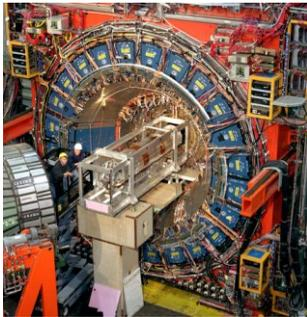
Fig 2: The Collider Detector at Fermilab that allowed the discovery of the top quark.
