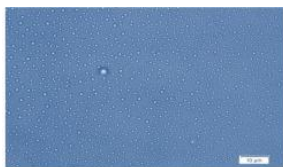
Bulk NBs can be visualized by optical microscopy (magnification of 1000 x) when contrasted with methylene blue dye in aqueous solution.
