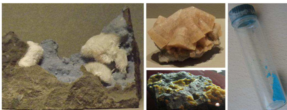
Figure 1. Natural and synthesized nanoporous materials: Mordenite (left), chabazite (center top), and stilbite (center bottom) from the Smithsonian Institution National Museum of Natural History and Cu-BTC (right) from Centre for Surface Chemistry and Catalysis (KU Leuven).
