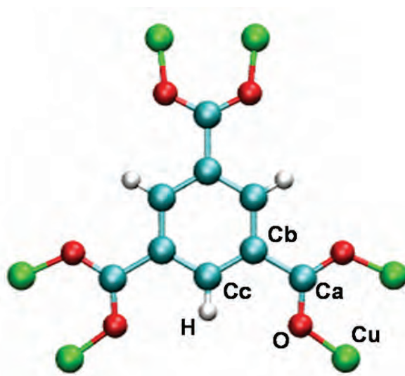
Figure 4.2. The crystallographically different atoms in Cu-BTC as defined in this work. We consider the following types of carbon atoms: Ca, linked to two oxygen atoms; Cb, linked to other three carbon atoms; Cc, linked to one hydrogen atom.
